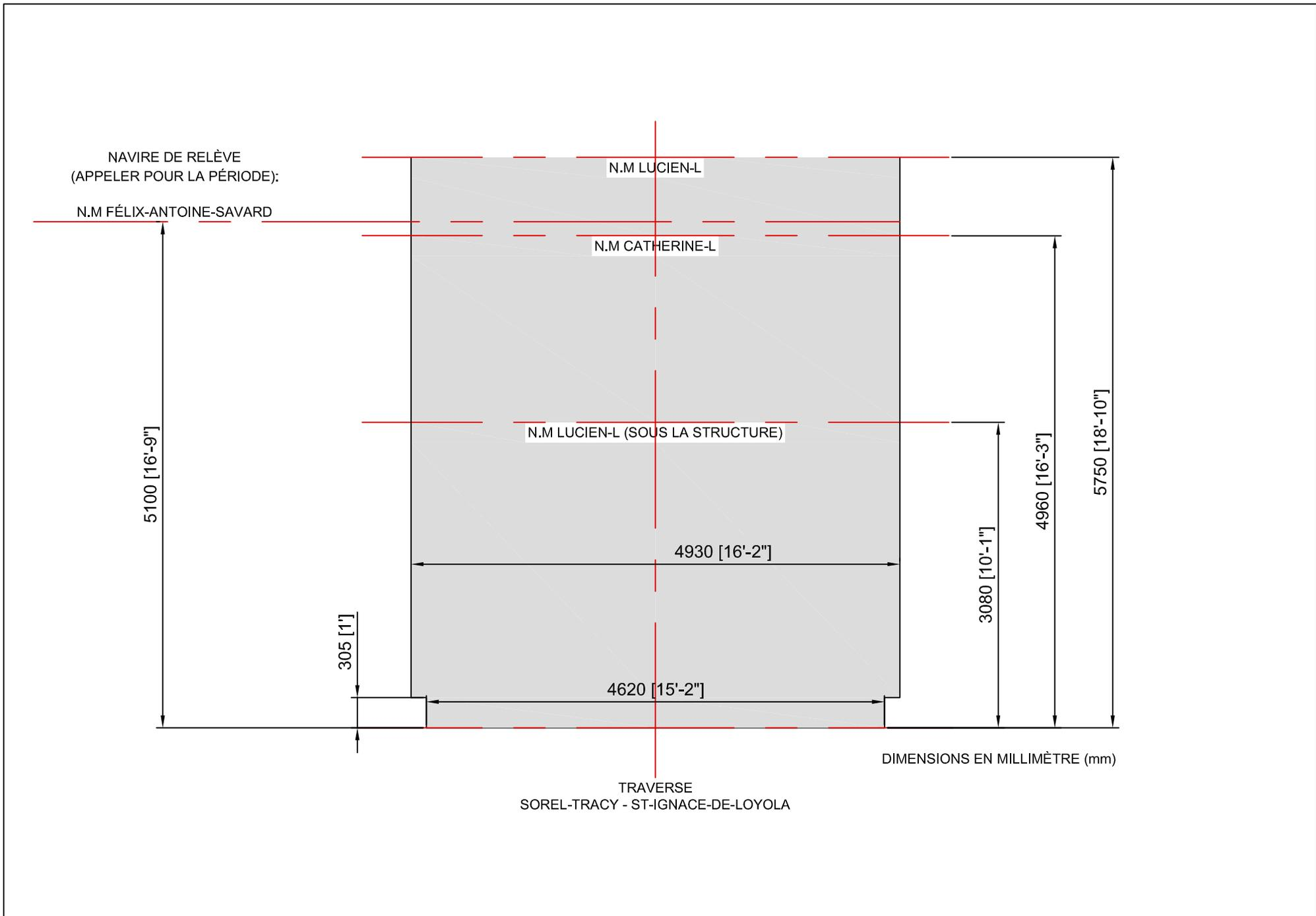
GABARIT MAXIMAL DE LA TRAVERSE FLUVIALE
